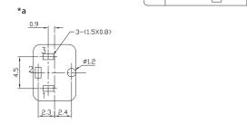
\*a printed circuit board layout, components side view
